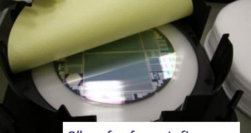
8" wafer from *Infineon* World largest Si detector
